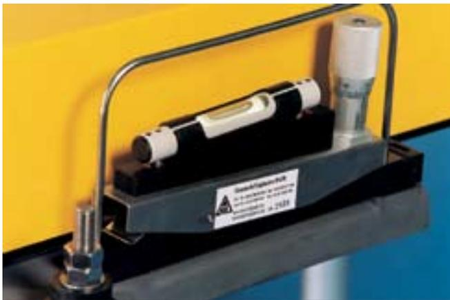
*Clinometer - No need to remove cover to fit clinometer.*
