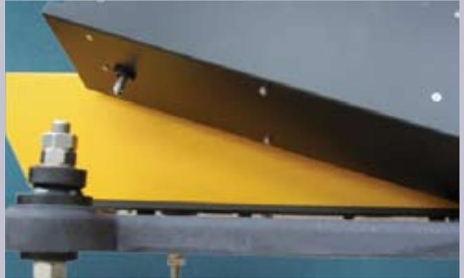
*Interchangeable PAPI Projectors - Research Engineers PAPI projectors are secured to the base frame by three, quarter turn DZUS quickly detachable fasteners. Workshop service and maintenance in accordance with ICAO RSM-9 is practicable.*
